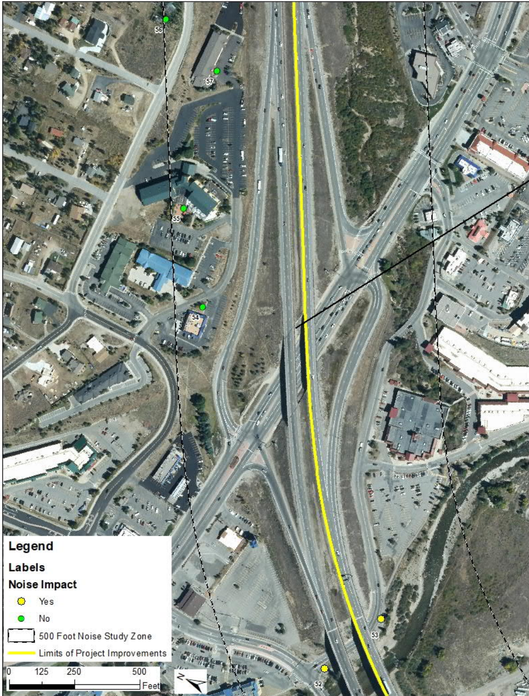
Figure 5C Roadways and Receiver Noise Levels for Design Year (2045) Proposed Action (Impacts Identified)
