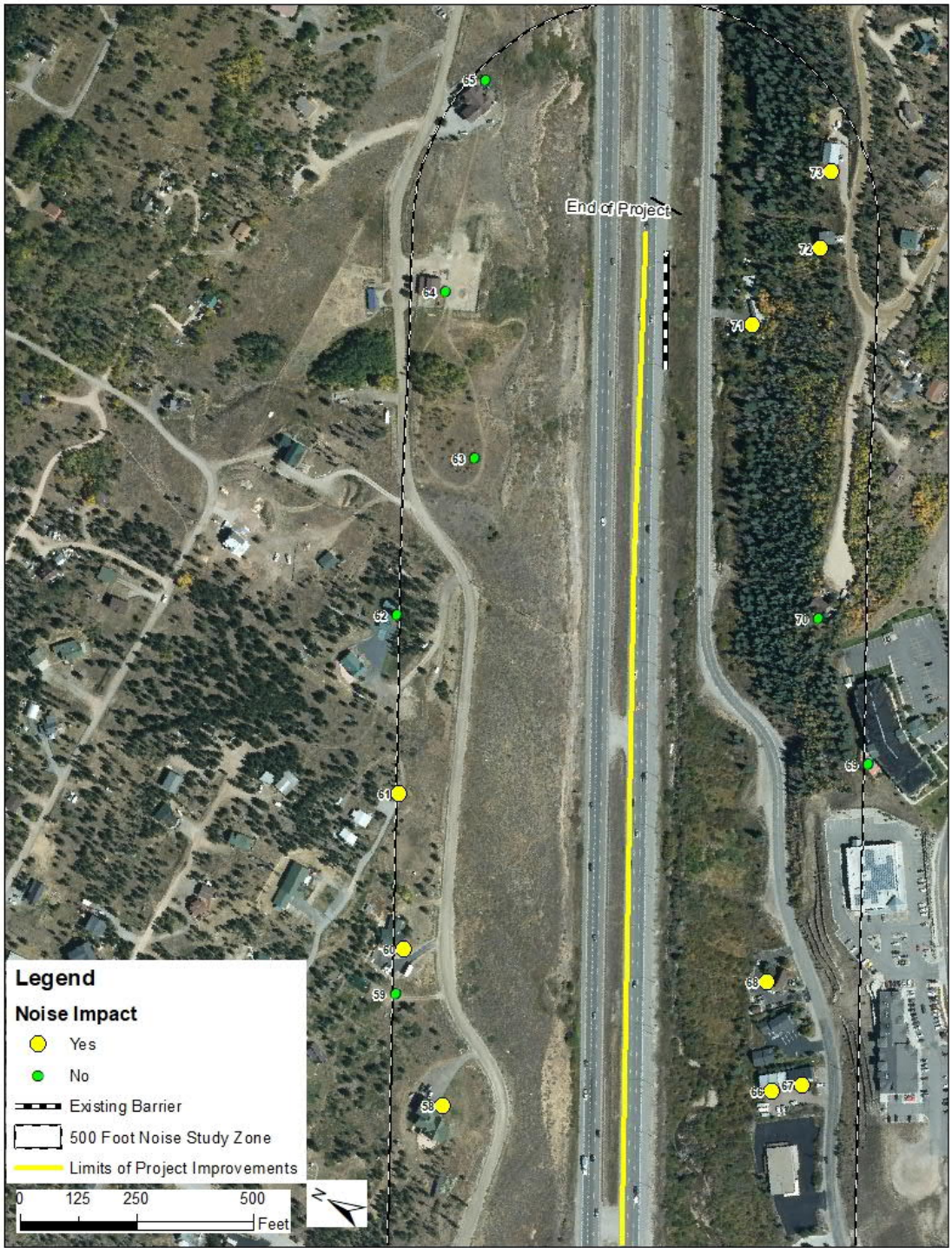
Figure 5D Roadways and Receiver Noise Levels for Design Year (2045) Proposed Action (Impacts Identified)
