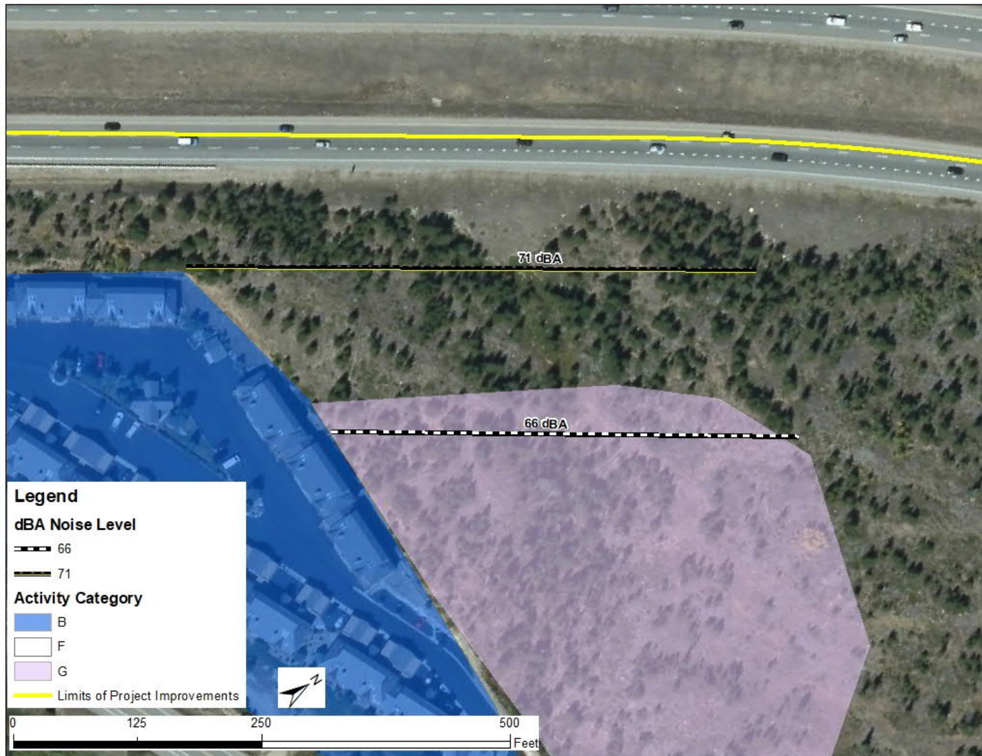
Figure 7 Interstate 70 EB Auxiliary Lane Noise 71 and 66 dBA Contours in Activity Category G Location
