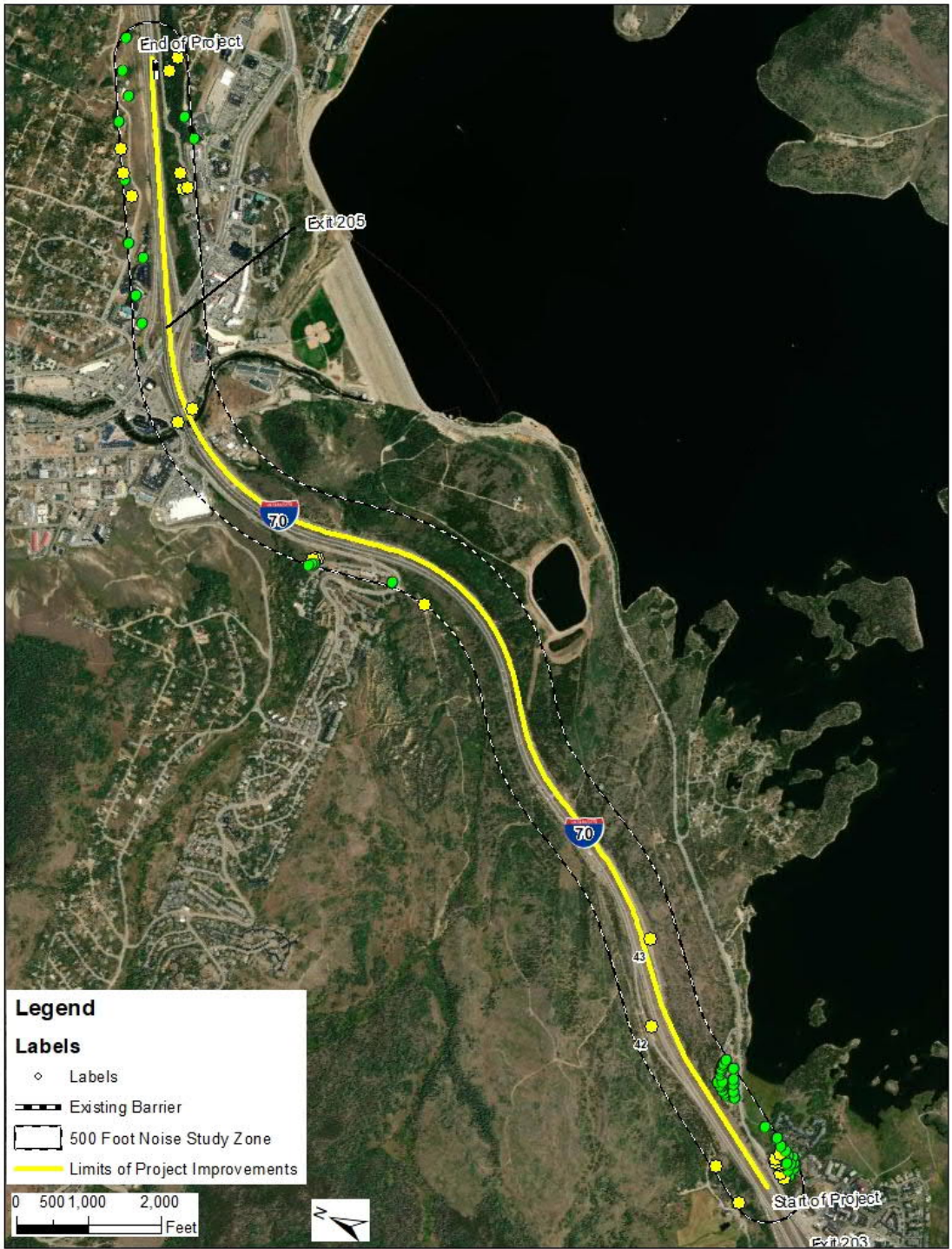
Figure 5 Roadways and Receiver Noise Levels for Design Year (2045) Proposed Action (Impacts Identified)
